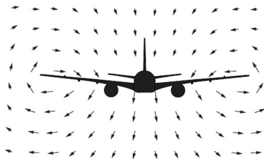
Figure 7 : Upwash / Downwash Effect
